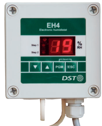
EH4 and standard room sensor IP65. Room sensor: low voltage 3 m. Optional: 25 m low voltage RJ9 extension cable (50 m maximum)
