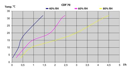
Specific energy consumption (SEC): 0,58 kWh/l at 20°C & 60% RH
